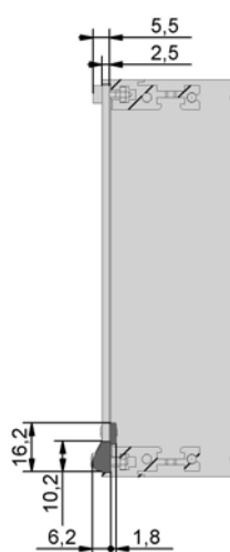
Side view, bottom-hinged / side-hinged with hinge extrusion
