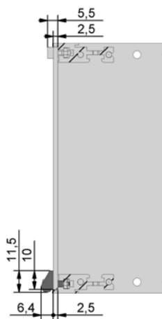
Side view, bottom-hinged / side-hinged with hinge element
